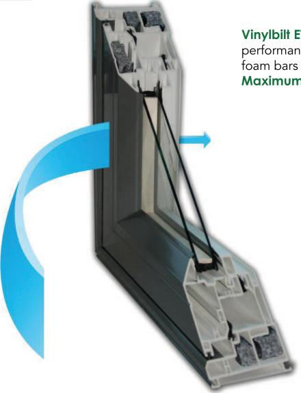
Vinylbilt ETI foam system combines the performance of engineered insulating rigid foam bars with dead air space to achieve Maximum thermal insulation
